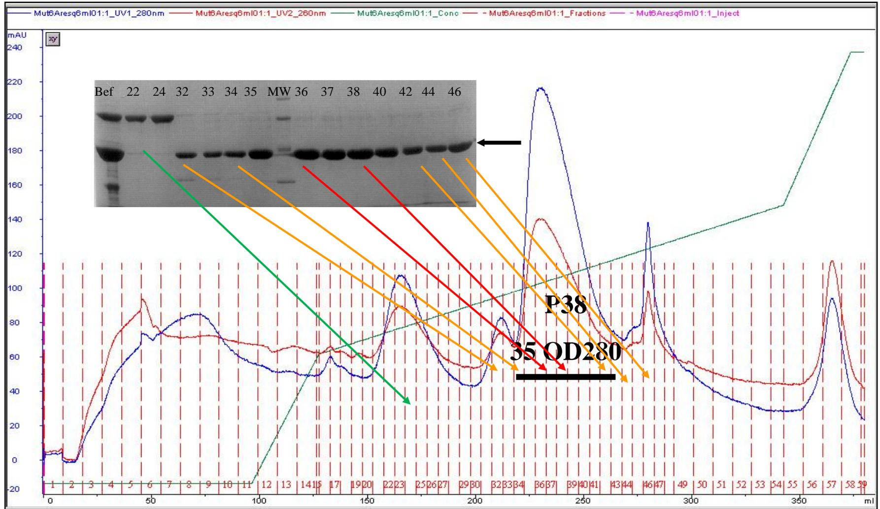
60 OD 280nm P38 after Ni-NTA and dialysis ON vs buffer A. Load on Resource Q-30 6ml column. Wash with 10cv 50mM NaCl buffer. Elute with gradient 5cv 50-300mM + 40cv 300-750mM + 5cv 750-1000mM NaCl
