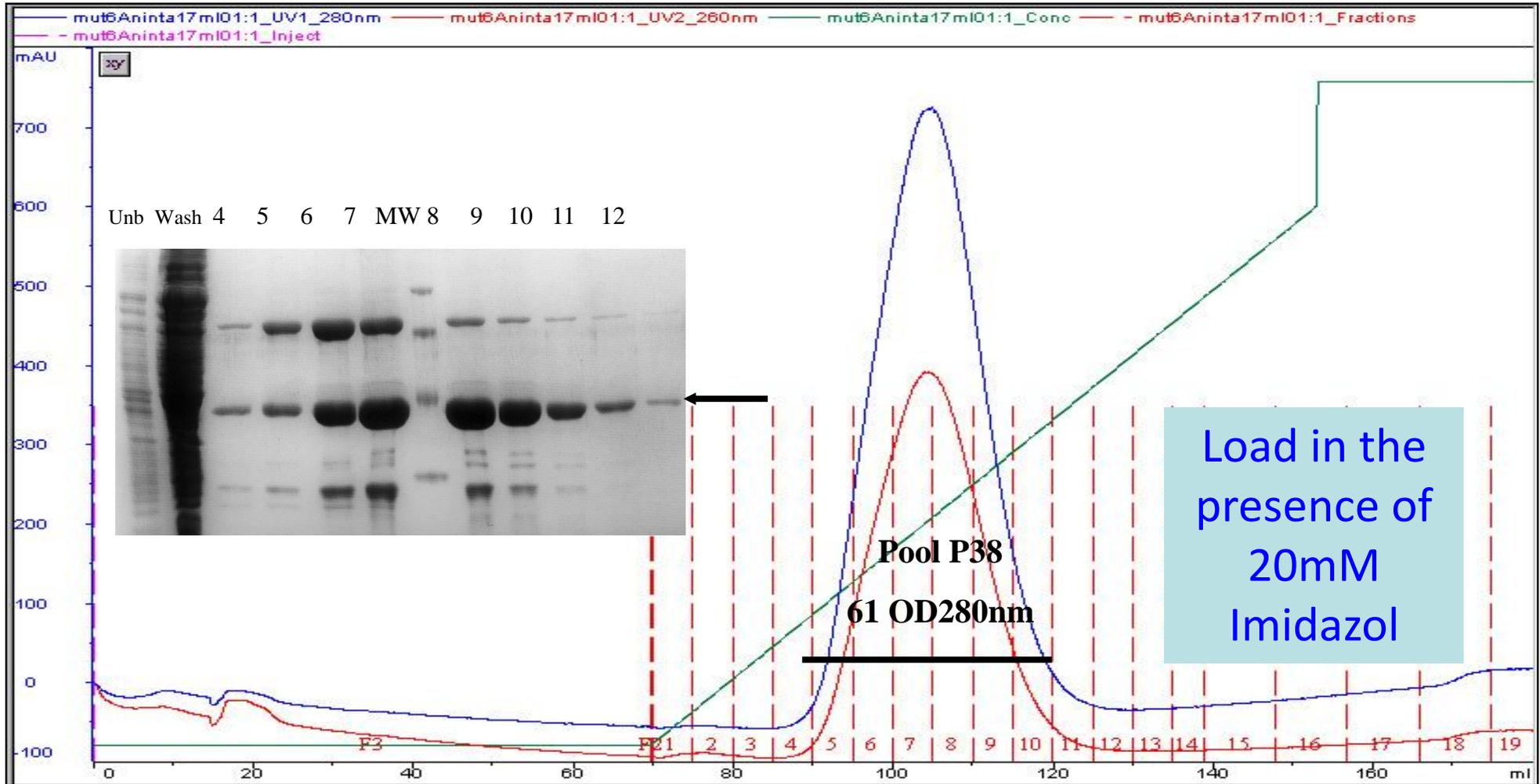
100gr cells (6L culture). Cell disruption with Mountain Goulin in 900ml lysis buffer. Batch binding to 15ml Ni-NTA 90min 4°C in the presence of 20mM Imidazol. Wash with 20mM Imidazol buffer and elution with 5cv gradient 20-250mM Imidazol.
